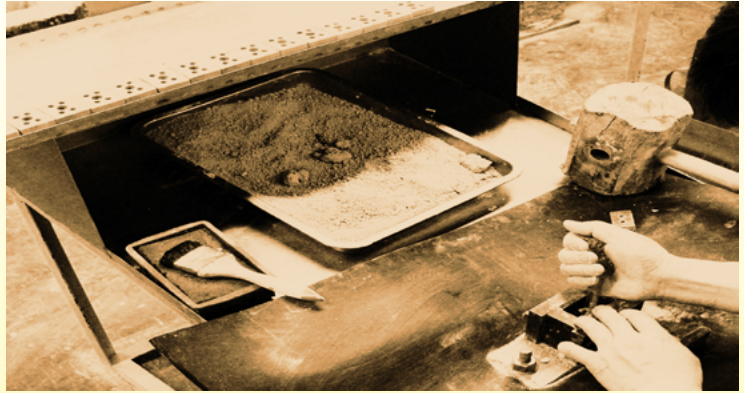
Porcelain Terminal Blocks Hand Made by Hammer Pressing: Manual Filling of Wet Granulate (Private Collection) Drying of Electric Porcelain After Pressing (Private Collection)
